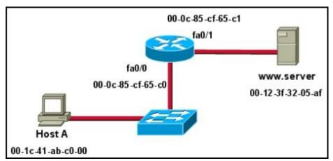
Refer to the exhibit. Assuming that the network in the exhibit is converged meaning the routing tables and ARP tables are complete, which MAC address will Host A place in the destination address field of Ethernet frames destined for http://www.server?
