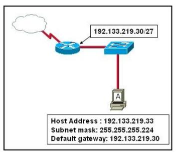
Refer to the exhibit. Host A is connected to the LAN, but it cannot get access to any resources on the Internet. The configuration of the host is shown in the exhibit. What could be the cause of the problem? The host subnet mask is incorrect.
