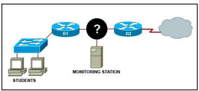
Refer to the exhibit. A network administrator has decided to use packet capture software to evaluate all traffic from the student subnet on the way to the Internet. To ensure that all packets are captured, what network device should be used to connect the monitoring station to the network between R1 and R2?
