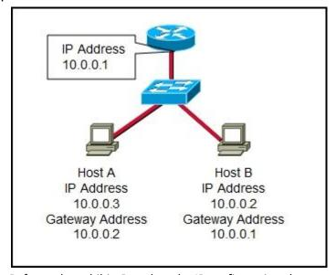
Refer to the exhibit. Based on the IP configuration shown, what would be the result of Host A and Host B attempting to communicate outside the network segment?
