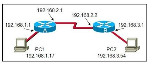
Refer to the exhibit. What destination IP address will PC1 place in the header for a packet destined for PC2?
