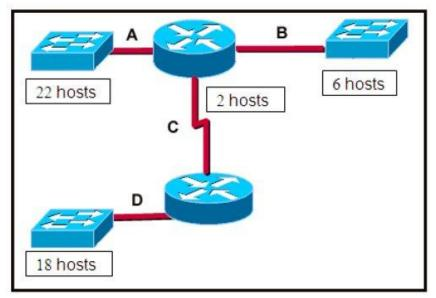
Refer to the exhibit. A network technician has been allocated the 192.168.1.0/24 private IP address range for use in the network that is shown in the exhibit. Which subnet mask would be used to meet the host requirements for segment A of this internetwork?
